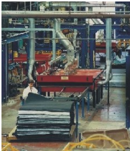
Pre Heat System for carpet sheets IRM
